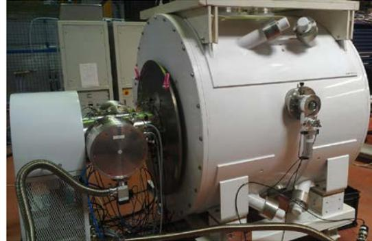
FIGURE 1. PMB-Alcen's ISOTRACE™ Super-Conducting Cyclotron for PET. The proton beam exit flange with gate valve is shown centre-right.
