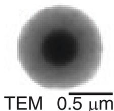
Figure 1: Transmission electron microscope (TEM) image of an anti-reflection coated, high-refractive index titania microsphere.
