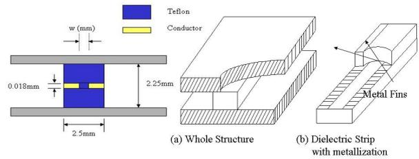
Fig. 4 Integration of NRD Guide and Slot Line
