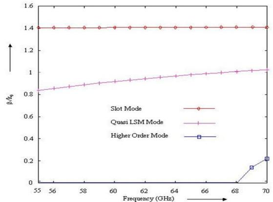
Fig. 5 Dispersion Characteristics of NRD Guide
