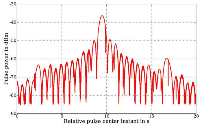
Fig. 5. Recorded datatake from a ground receiver showing the azimuth pattern.
