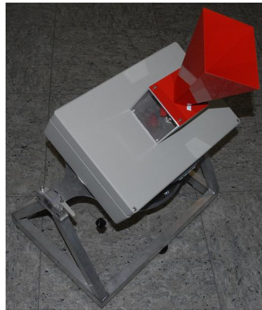
Fig. 3. Ground receiver. The housing can be rotated in steps of  $45^\circ$  to allow polarimetric characterization of the satellite.
