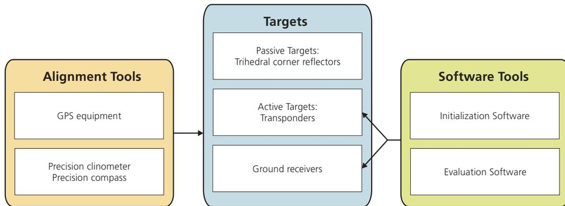
Fig. 1. Overview of the calibration ground equipment.
