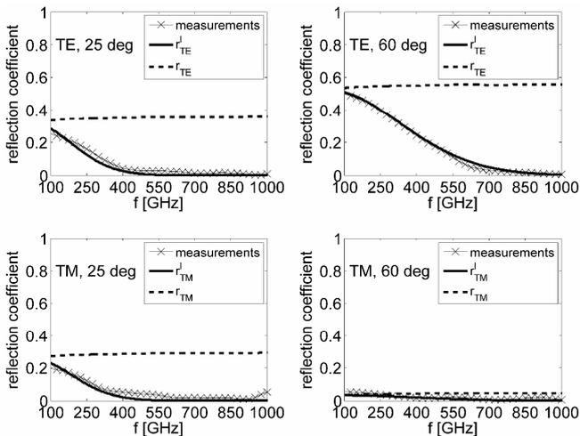
Fig. 3 Calculated magnitude of reflection coefficients  $r_{TE}$  and  $r_{TM}$  and of modified reflection coefficients  $r'_{TE}$  and  $r'_{TM}$  and direct reflection measurements of plaster sample in the frequency range from 100 to 1000 GHz for two angles of incidence of TE and TM polarized waves: 25 deg, 60 deg.
