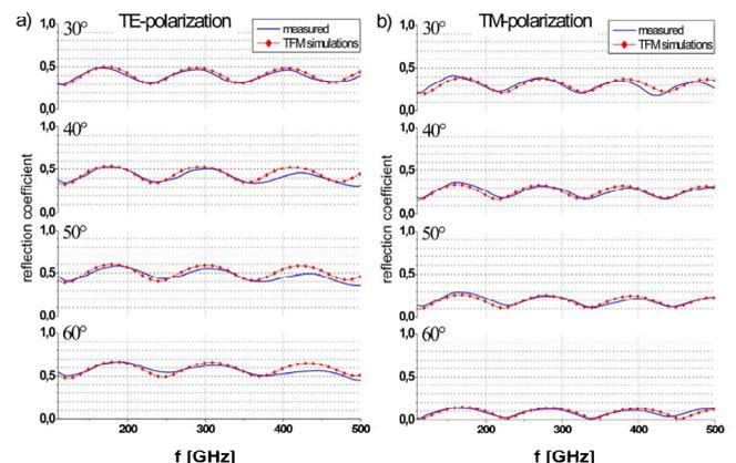
Fig. 5 Measured data (solid lines) and transfer matrix simulations (lines and symbols) of the frequency and angle dependent amplitude reflection coefficient of a white paint on plaster
