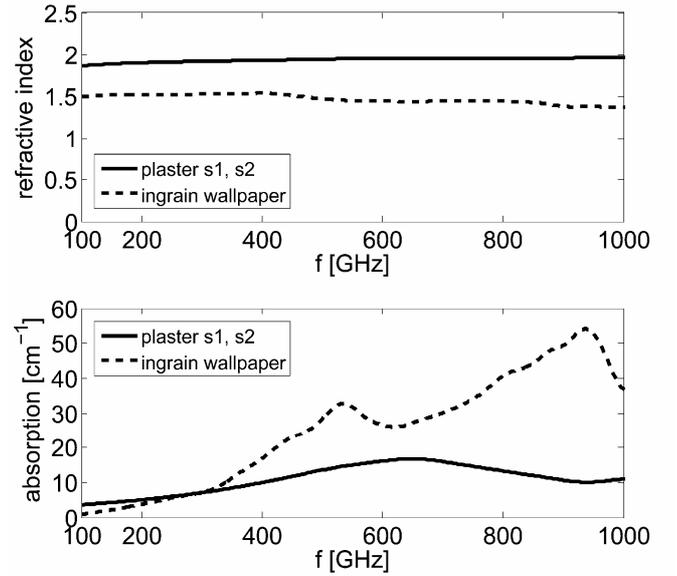
Fig. 1 Measurements of refractive index (top) and absorption coefficient (bottom) of the investigated concrete plaster sample.
