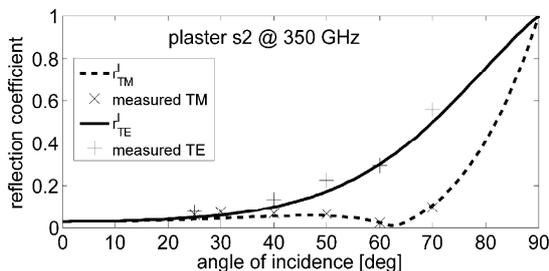
Fig. 4 Calculated magnitude of modified reflection coefficients  $r'_{TE}$  and  $r'_{TM}$  and direct reflection measurements of plaster sample for angles of incidence between 0 and 90 degrees at a frequency of 350 GHz for TE and TM polarized waves.
