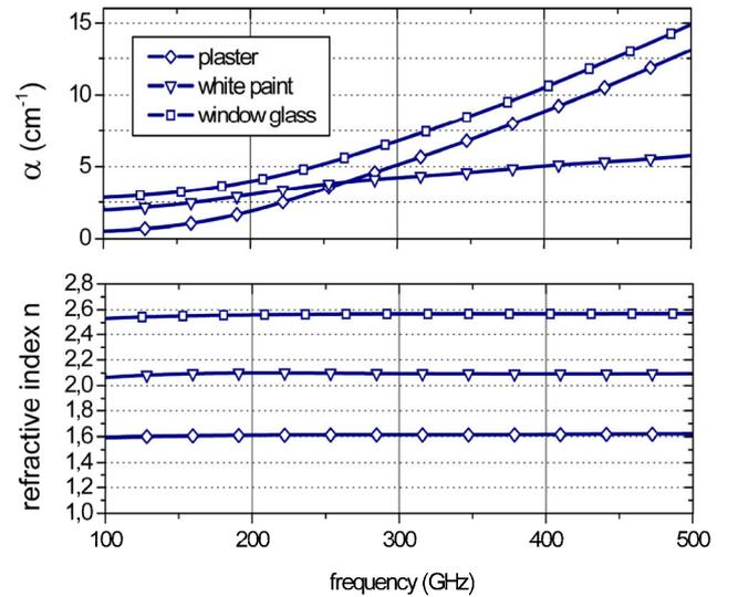
Fig. 2 Frequency dependent absorption coefficient  $\alpha$  and refractive index  $n$  of gypsum plaster and white paint.
