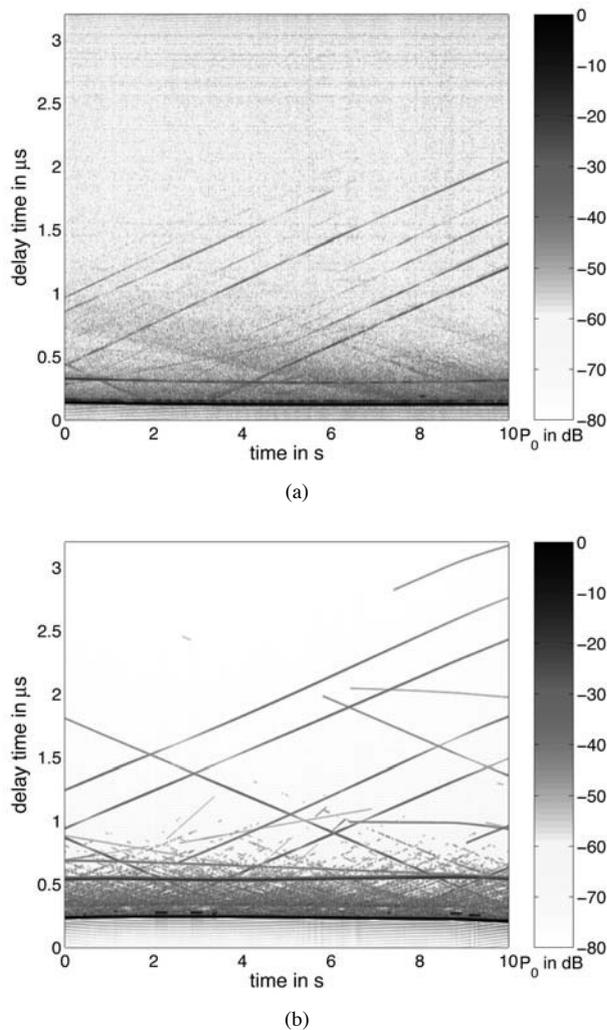
Fig. 8. Power delay profile for car-to-car communications in a motorway environment: measurement (a) and ray-tracing simulation (b)
