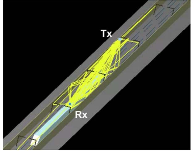
Fig. 1. High-speed train in a noise barrier scenario. The yellow lines represent the simulated propagation rays.
