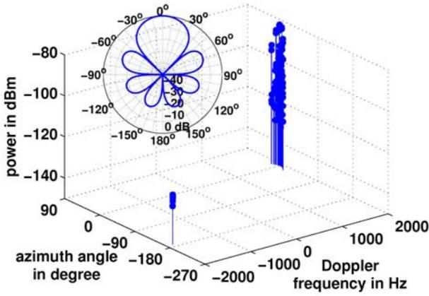
Fig. 3. Path power versus Doppler frequency and azimuth angle (DoA) for a representative snapshot using a directional train antenna (azimuth pattern given in the upper left-hand corner)
