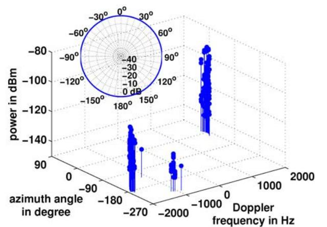
Fig. 2. Path power versus Doppler frequency and azimuth angle (DoA) for a representative snapshot using an omnidirectional train antenna (azimuth pattern given in the upper left-hand corner)
